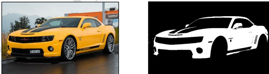
Figure 20: Colour mask to track yellow colour in the input image
